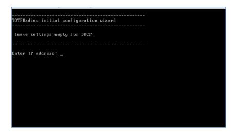
Enter IP address, Subnet mask and default gateway. After that, the machine will continue to boot up.
